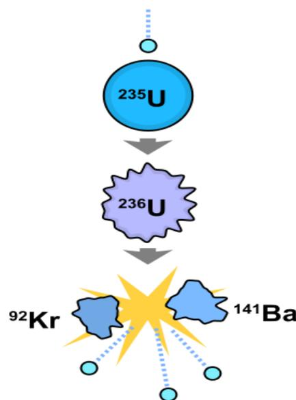
An induced fission reaction. A neutron is absorbed by a uranium-235 nucleus, turning it briefly into an excited uranium-236 nucleus, with the excitation energy provided by the kinetic energy of the neutron plus the forces that bind the neutron. The uranium-236, in turn, splits into fast-moving lighter elements (fission products) and releases three free neutrons. At the same time, one or more "prompt gamma rays" (not shown) are produced, as well.
