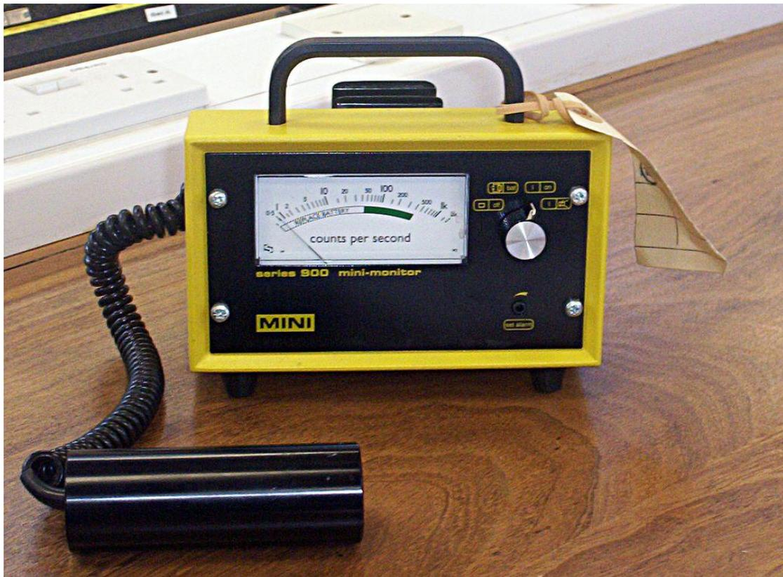
The Geiger-Müller tube is filled with an inert gas such as helium, neon, or argon at low pressure, to which a high voltage is applied. The tube briefly conducts electrical charge when a particle or photon of incident radiation makes the gas conductive by ionization. The ionization is considerably amplified within the tube by the Townsend Discharge effect to produce an easily measured detection pulse, which is fed to the processing and display electronics. This large pulse from the tube makes
