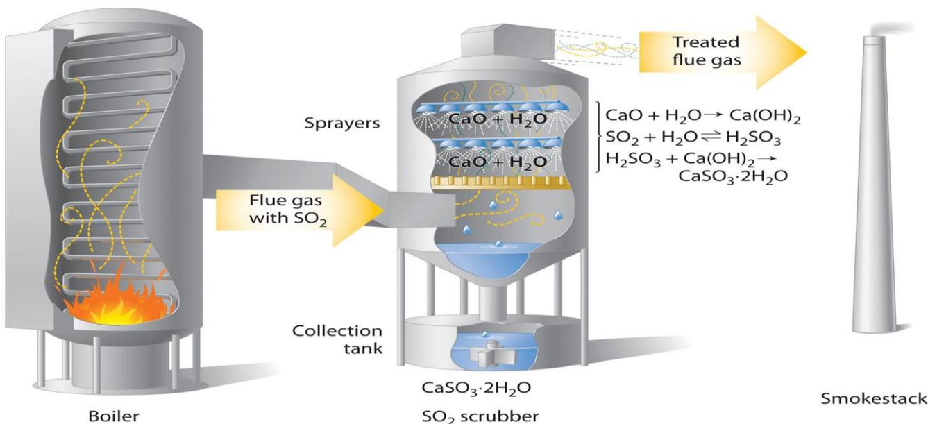
Fig( 1): Schematic Diagram of a Wet Scrubber System .
